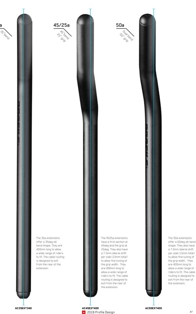
shape. They also have a 7.5mm lateral shift per side (15mm total) to allow fine tuning of the grip width. They are 400mm long to allow a wide range of riders to fit. The cable routing is designed to exit from the rear of the extension.
